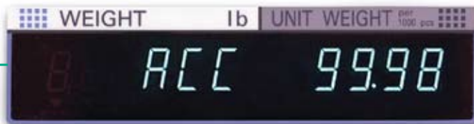
The DC-190 lets you know the accuracy percentage of unit weights based on scale capacity.
